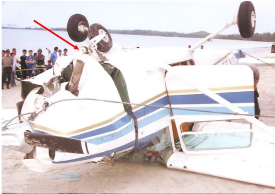
Figure 3: Arrow points to fractured nose landing gear
