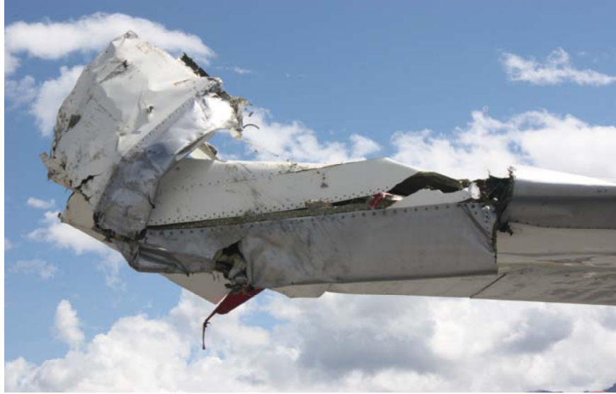
Figure 1: The damaged right wing tip
